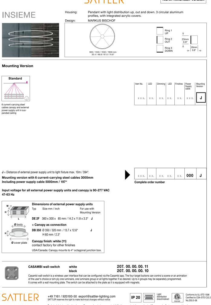
Technical data is subject to change. Errors and omissions excepted 1) Net lumen output: Losses due to diffusors and reflectors are considered. Lumen values refer to an ambient temperature of max. 35° Celsius / 95° Fahrenheit. 2) Weight of lights without remote technical unit or canopy.
